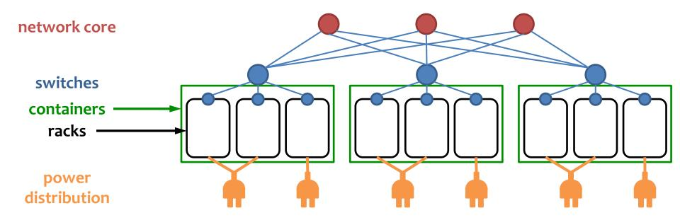
Complex fault domains: networking, power, cooling
